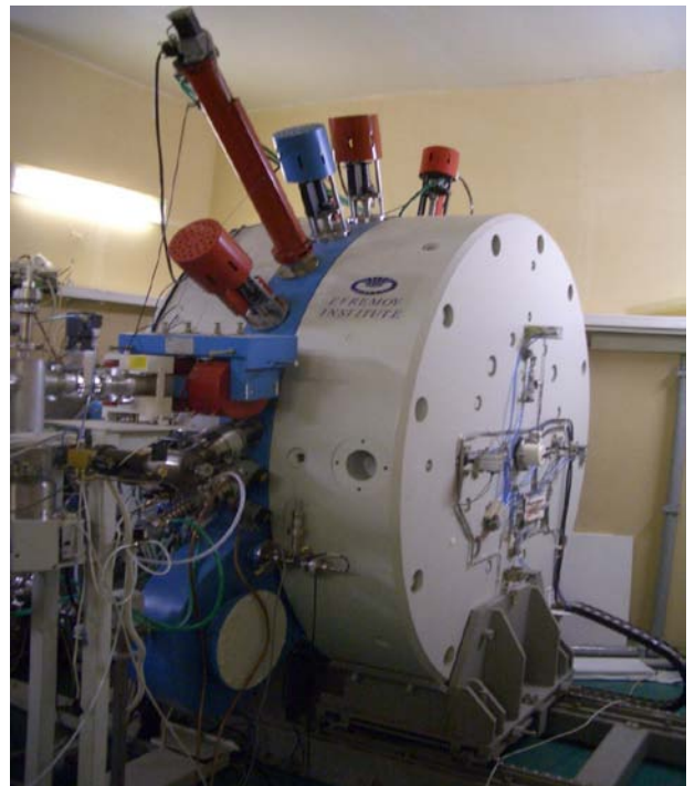
CC-18/9 Cyclotron, delivered to the Russian Research Center for Radiology and Surgical Technologies, Pesochny, St.Petersburg (2006)
