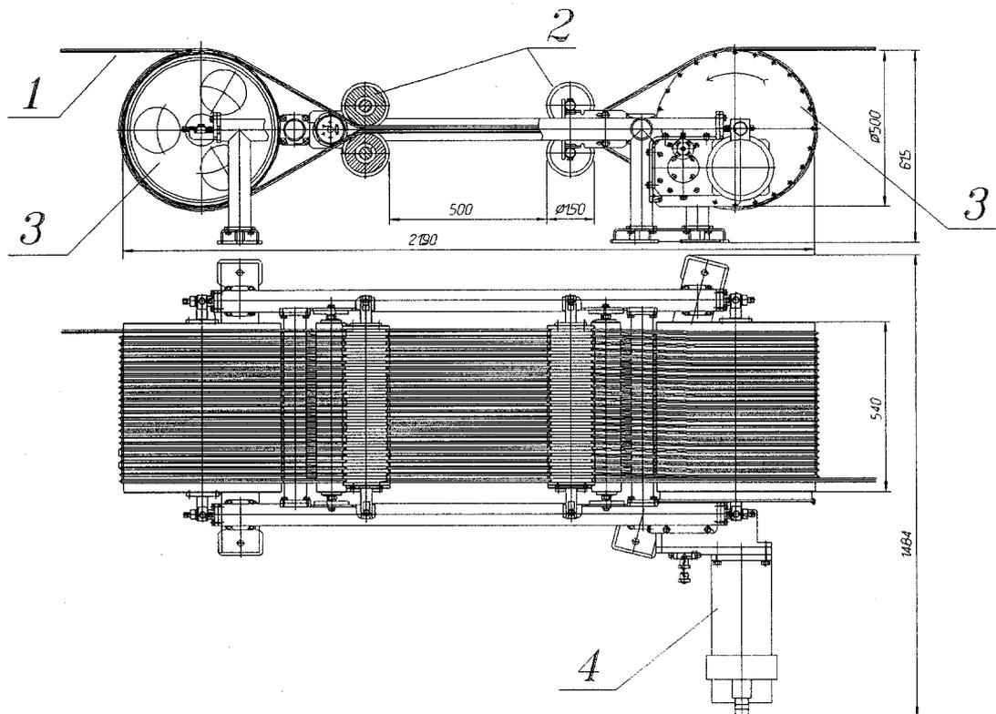
Figure 15: General view of the transport device. 1 - an irradiated object; 2 - guiding rolls; 3 - drums; 4 - drive
