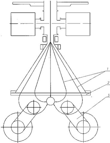
Figure 14: System of Circular Irradiation. *1-electron trajectory, 2-extraction window, 3-bending magnets*
