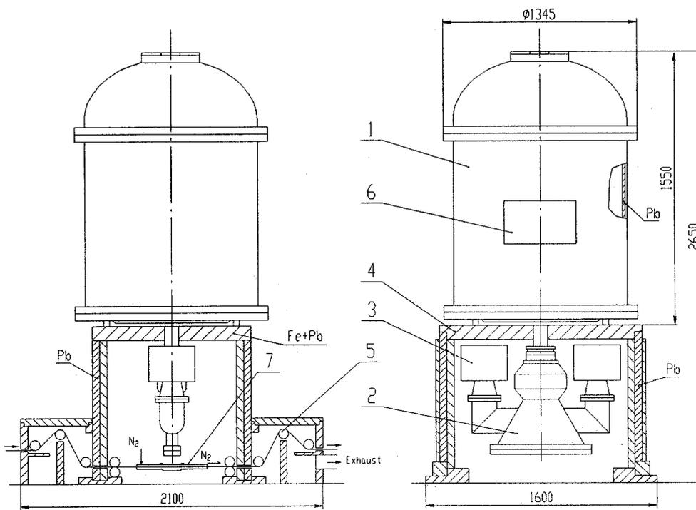
Figure 17: ELV-0.5 accelerator in local radiation protection. 1 - tank, 2 - extraction device, 3 - vacuum pumps, 4 - elements of protection, 5 - conveyor, 6 - admission of control and power supply cables, nitrogen chamber (for the processes required the irradiation in the inert medium)
