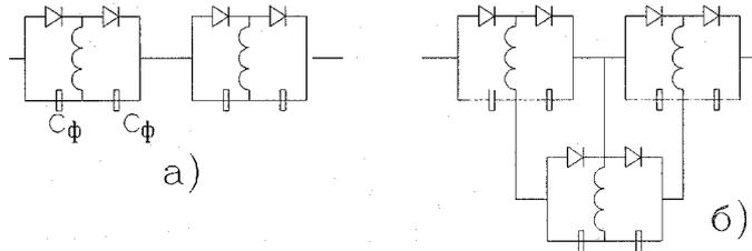
Figure 6: ELV rectifying section circuit and ways of their connection
