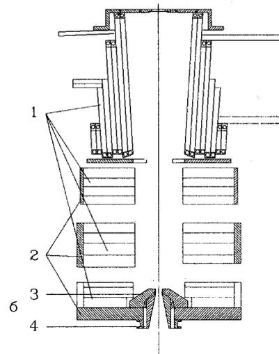
Figure 13: Vacuum system of an extraction device with an adiabatic compression of a beam. (1,2-tubes of high vacuum resistance, 3, 5-diaphragms, 4 - vacuum lines)
