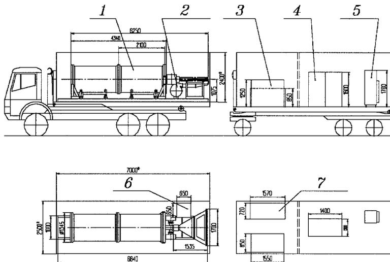
Figure 5: Transportable version of the ELV-6 accelerator. 1 - accelerator; 2 - foil cooling system; 6 - vacuum system; 7 - frequency converter
