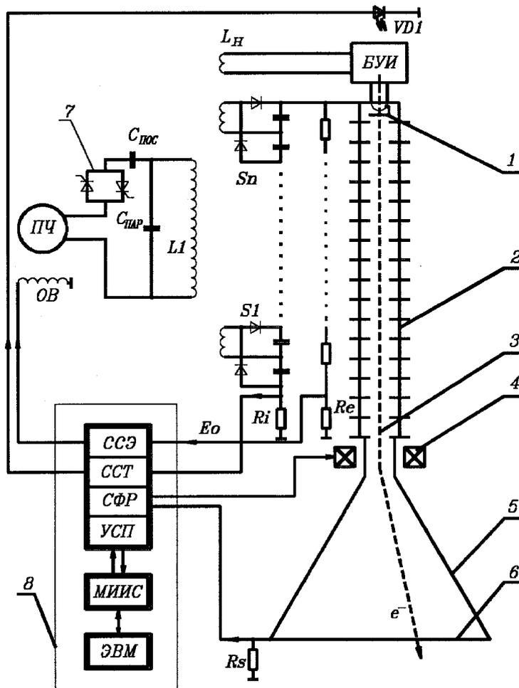
Figure 3: Simplified electric circuit of ELV accelerator. 1 - cathode of electron gun; 2 - accelerating tube; 3 - electron beam; 4 - coils of the raster formation system; 5 - extraction device; 6 - titanium foil; 7 - thyristor switch; 8 - control system (ESS-energy stabilizing system, CSS- current stabilizing system, RFS-raster formation system, MIMS-module information-measuring system, CC-Control Computer, PSCS-power supply control system). FC - frequency converter, ICU-injector control unit
