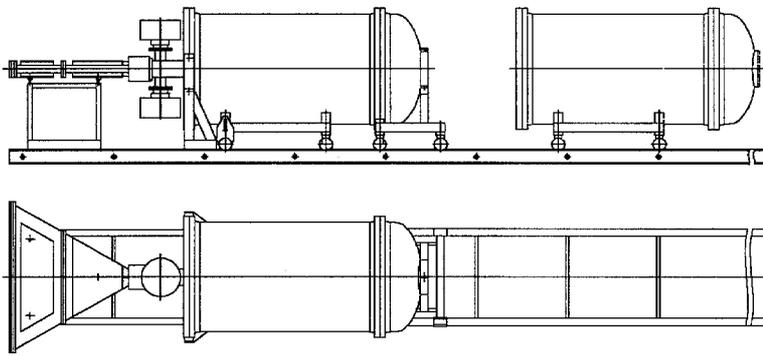
Figure 4: ELV-4 accelerator. Horizontal version. On the basis of this version the ion implanter has been developed at the Institute
