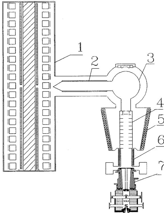
Figure 19: “Torch-accelerator”: 1 - the source of accelerating voltage, 2 - gas feeder, 3 - injector control system, 4 - accelerating tube, 5,6,7 - the system of raster formation and vacuum system
