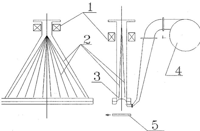
Figure 8: Schematic diagram of extraction device with a foil window. 1 - scanning electromagnets, 2 - beam trajectories; 3 - foil of extraction window; 4 - foil cooling fan; 5 - movable target
