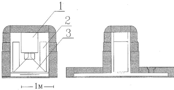
Figure 16: Local protection of the ELV-mini accelerator. 1 - accelerator, 2 - vacuum pumps, 3 - extraction device.
