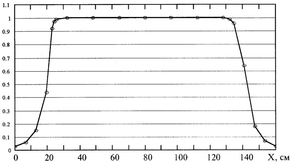
Figure 9: Typical distribution of current linear density under the frame of extraction window at an energy of electrons of 1.5 MeV
