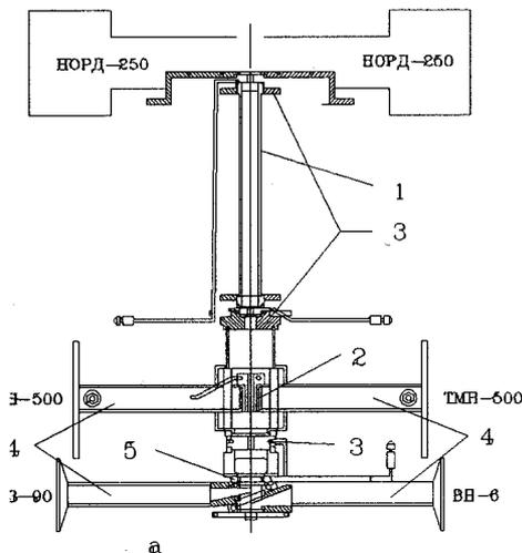
Device for the extraction into air of an adiabatically compressed intense electron beam:
