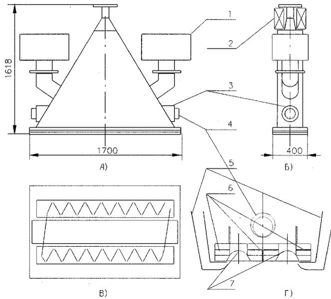
Figure 10: Two-window extraction device: 1 - magnetodischarge pumps, 2 - coils and cores of the beam scanning system, 3 - protection cylinder flange, 4 - protection cylinder, foil blow, 5 - air jet cooling, 6 - frame for fixation of foil, 7 - extraction foils.
