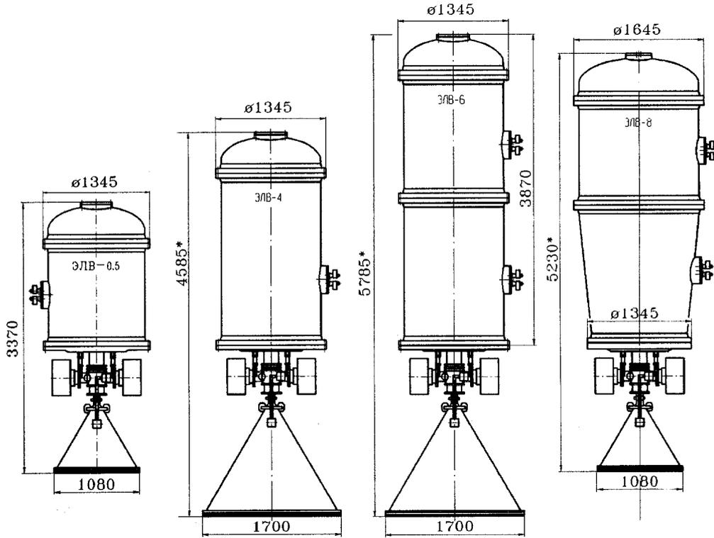
Figure 1: Overall dimensions of ELV-type accelerators
